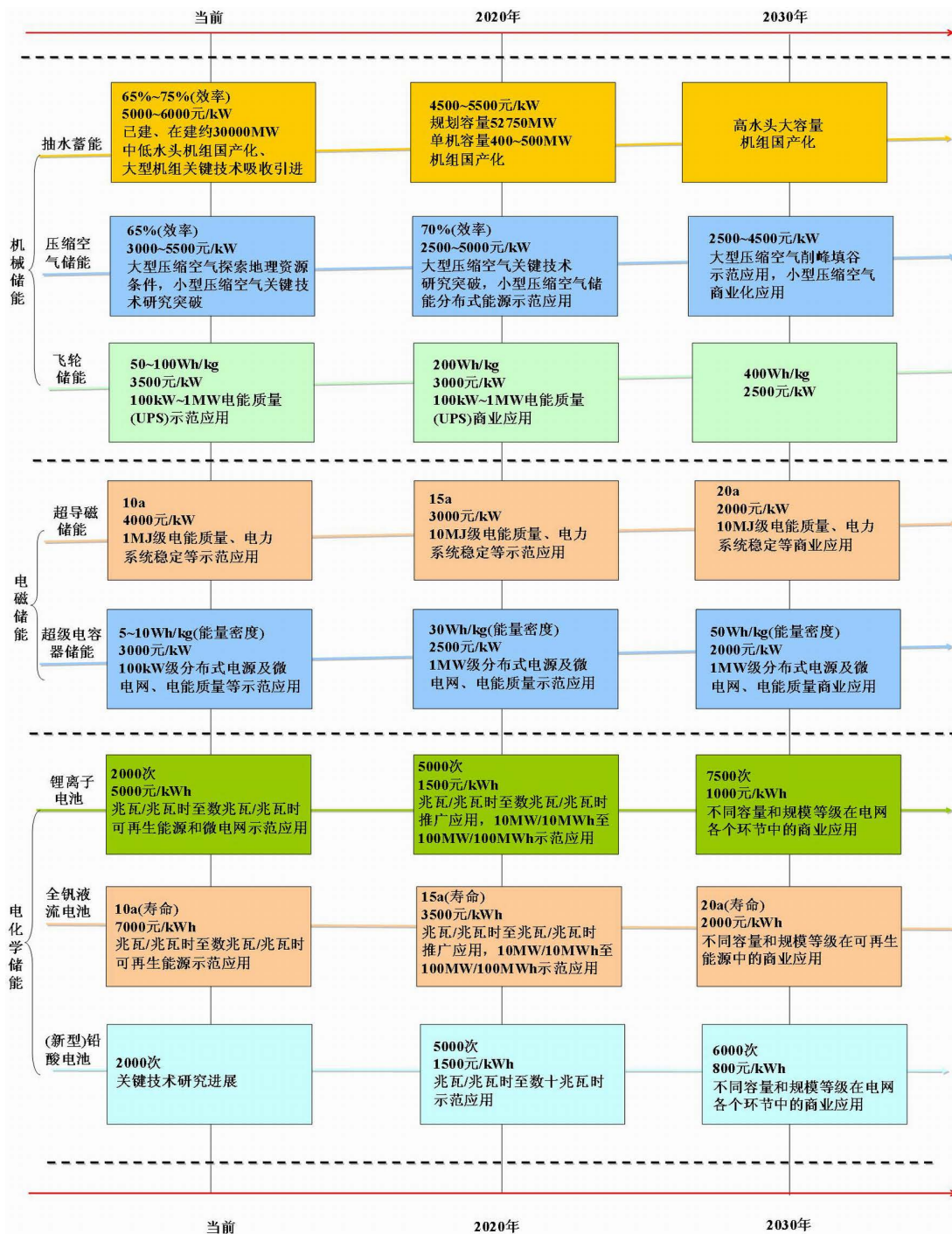
Figure 2. The development and application roadmap for large-scale energy storage technologies in China 图 2. 大规模储能技术在中国发展及应用的路线图
