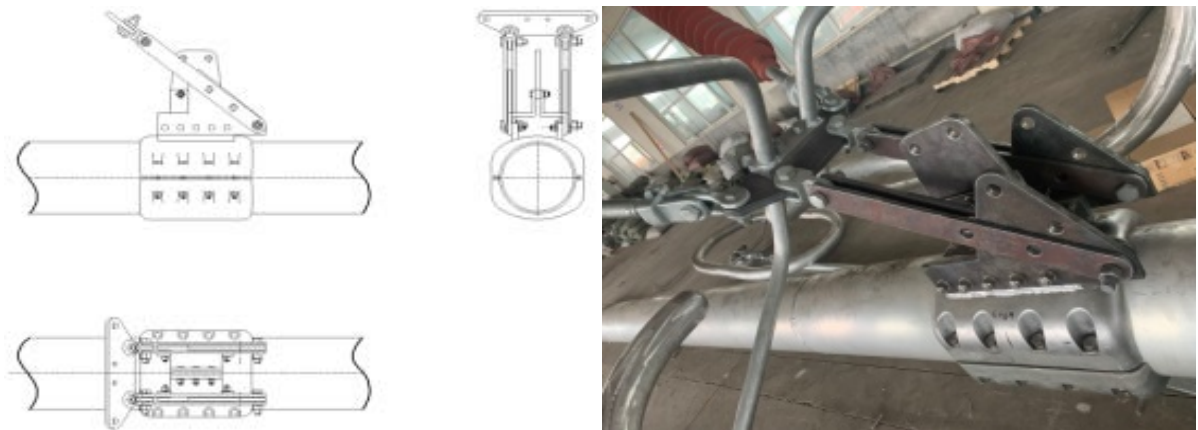
Figure 9. Structure diagram of height adjustment mechanism
