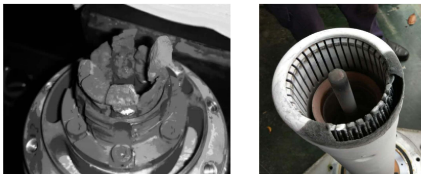
Figure 7. The contact is severely ablated 图 7. 触头严重烧蚀
