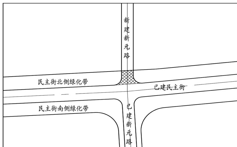
Figure 4. New road intersection does not meet overall land use planning overall land use planning 图 4. 新建道路交叉口不符合土地规划
