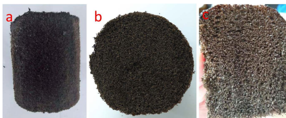
Figure 2. The macro images of foaming materials with Bayberry bark pre-concentration: (a) the whole foaming materials; (b) section diagram in perpendicular to foaming direction; (c) section diagram in parallel to the foaming direction 图 2. 杨梅树皮预缩液发泡材料实物图: (a) 发泡材料实物; (b) 发泡材料横向截面图; (c) 发泡材料纵向截面图
