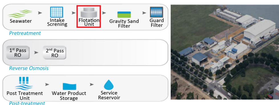
Figure 6. SingSpring desalination plant process at Tuas Singapore
