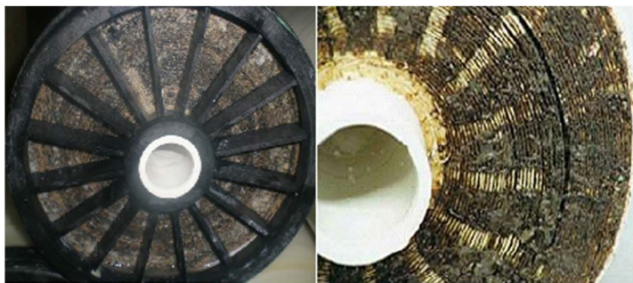
Figure 3. Algae microbial pollution of seawater desalination on reverse osmosis membrane 图 3. 海水淡化反渗透膜的藻类污染
