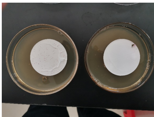
Figure 1. Experimental results of Streptococcus faecalis culture medium (reaction time: 1 min, raw water on the left)
