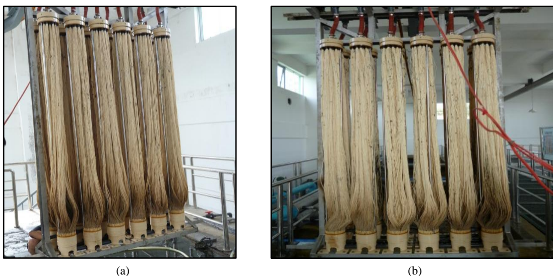
Figure 12. The membrane assembly after artificial physical maintenance 图 12. 人工物理维护后的膜组件
