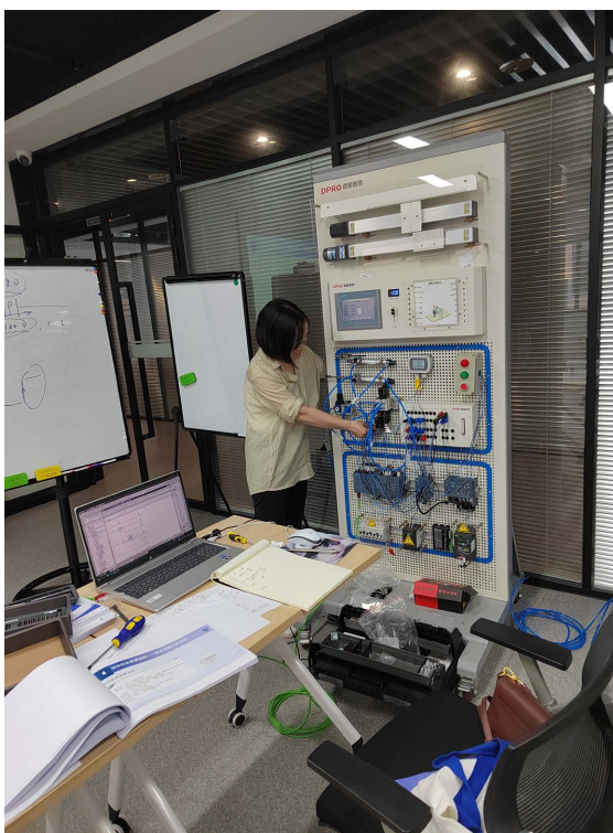
Figure 4. The enterprise teacher is checking the student's connection line
