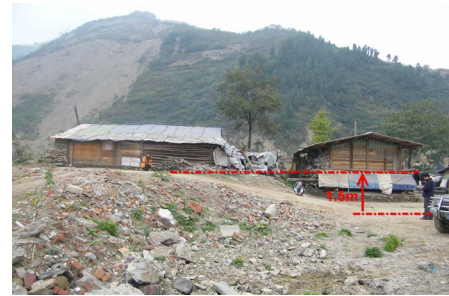
Photo 5. NB-5 thrust dextral, vertical dislocation 1.5 m, horizontal dislocation 1.3 m, Mirror to the North 照片 5. 南坝-5 逆冲右旋, 竖向位错 1.5 m, 水平位错 1.3 m, 镜向北
