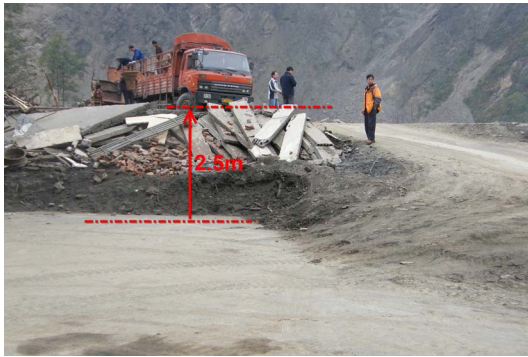
Photo 1. NB-1 thrust dextral, vertical dislocation 2.5 m, located at Jiankang of Nanba Town, Mirror to N50°W 照片 1. 南坝-1 逆冲右旋, 竖向位错 2.5 m, 位于南坝镇建康村, 镜向 N50°W
