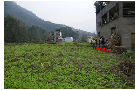
Photo 4. NB-4 apparent uplift in field, vertical dislocation 0.5 m, located at Mowan village, Mirror to N40°E 照片 4. 南坝-4 庄稼地明显抬升, 竖向位错 0.5 m, 位于磨湾村, 镜向 N40°E
