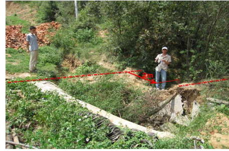
Photo 3. NB-3 dextral strike-slip, strike-slip 2 m, located at Wenjiaba of Nanba Town, Mirror to N80°W 照片 3. 南坝-3 右旋走滑, 走滑量为 2 m, 位于南坝文家坝村, 镜向 N80°W
