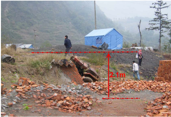
Photo 2. NB-2 thrust dextral, vertical dislocation 2.1 m, located at a hill near Shika gas station, Mirror to N20°W 照片 2. 南坝-2 逆冲右旋, 竖向位错 2.1 m, 位于石坎加油站后山, 镜向 N20°W
