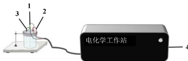
Figure 1. Schematic diagram of the three-electrode system; 1) Working electrode; 2) Platinum sheet electrode; 3) Saturated calomel electrode; 4) Electrochemical workstation
