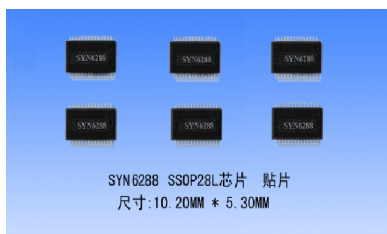
Figure 7. The packaging information of SYN6288 speech synthesis chip 图 7. SYN6288 语音合成芯片封装信息
