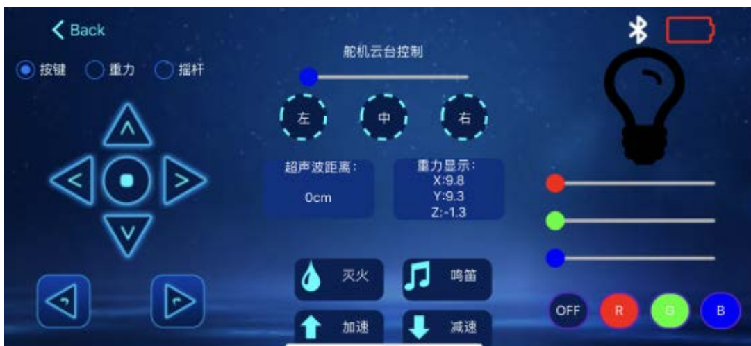
Figure 6. Bluetooth control interface of the Android App
