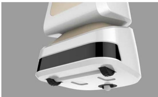
**Figure 4.** Universal wheels and navigation module at the bottom of the fuselage
