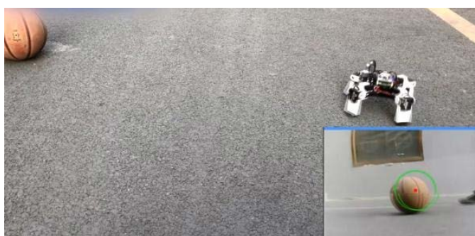
Figure 8. Color recognition and following function test effect diagram 图 8. 颜色识别与跟随功能测试效果图
