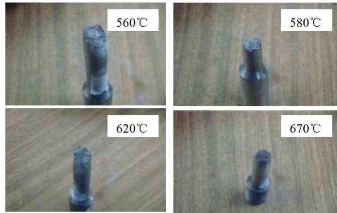
Figure 3. Tensile specimen macroscopic fracture at different tempering temperatures
