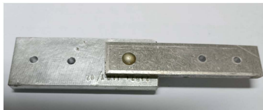
Figure 10. Shear test riveting photograph 图 10. 剪切试验铆接照片
