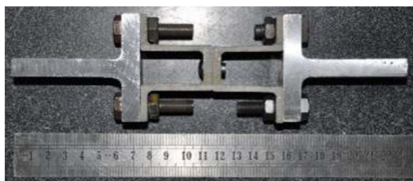
Figure 12. Photo of riveting for pull out test 图 12. 拉脱试验铆接照片
