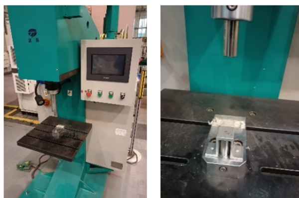
Figure 8. Riveting test piece was prepared by servo riveting machine
