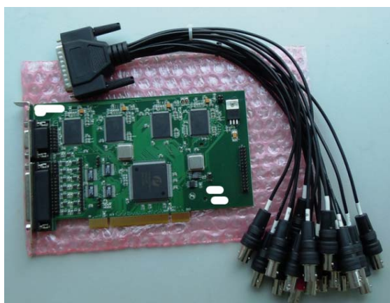
Figure 4. A photo of the A01 video capture card 图 4. A01 视讯撷取卡成品图
