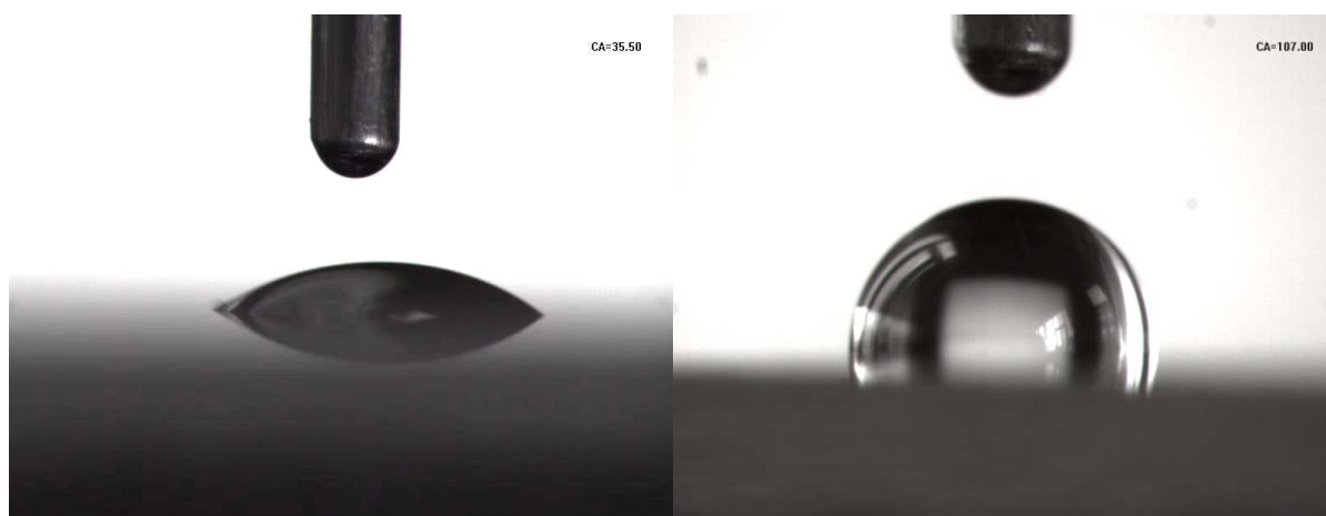
Figure 1. Comparison diagram of surface hydrophobic treatment of medicinal glass bottle before (a, \theta = 35.5^\circ ) and after treatment (b, \theta = 107^\circ )
