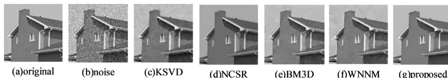
Figure 4. \sigma = 50 House image denoising effect comparison chart USES a variety of algorithm 图 4. \sigma = 50 时 House 图像使用多种算法去噪效果比较图
