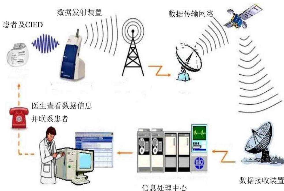
Figure 1. The component and working network of cardiac remote monitoring; (Adapted an revised with permission from: www.biotronik.com )
