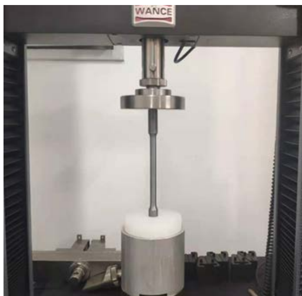
Figure 2. The electronic mechanical machine pushes away the prosthesis and base
