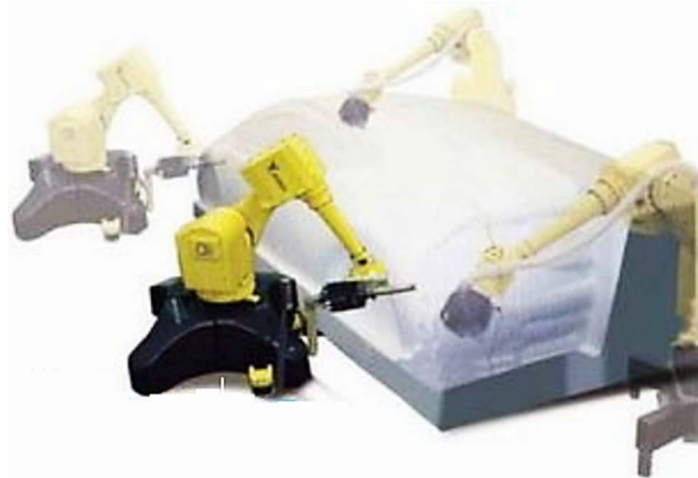
Figure 5. Group machining schematic diagram of large parts 图 5. 大型零件的群体加工示意图
