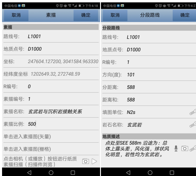
Figure 4. Properties box of field sketch and routing (R process) on the handheld
