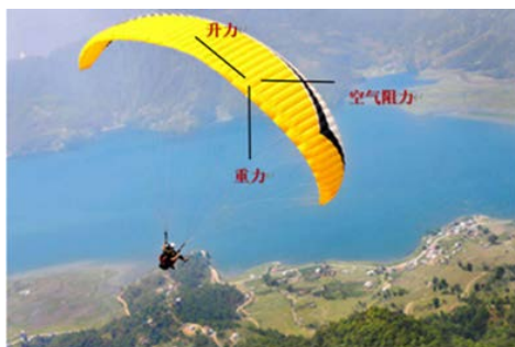
Figure 2. Force analysis diagram of paraglider 图 2. 滑翔伞受力分析图
