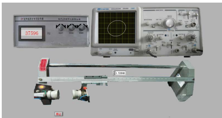
Figure 2. The front panel of experiment on measuring sound velocity in air 图 2. 测空气中声速实验虚拟前面板
