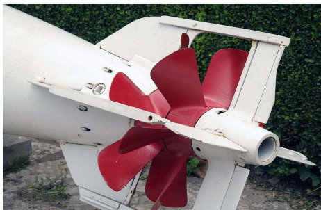
Figure 3. Twin propellers at the tail of the torpedo 图 3. 鱼雷尾部的双螺旋桨
