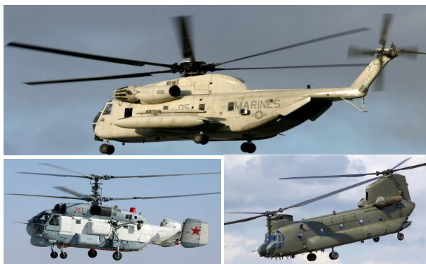
Figure 2. From helicopters with tails to twin-rotor helicopters 图 2. 从带尾翼的直升机到双旋翼直升机
