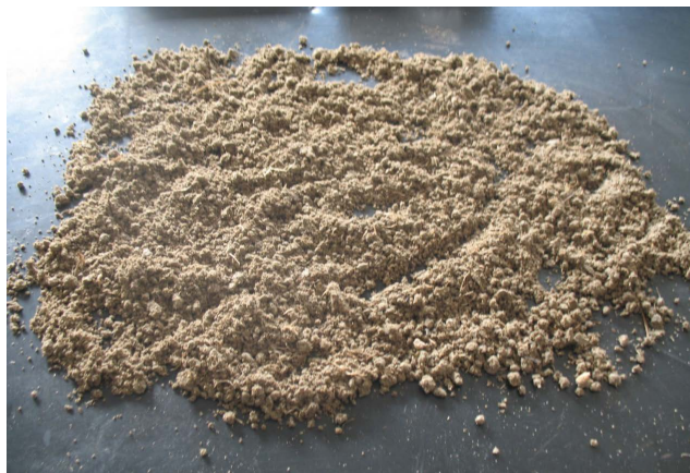
Figure 2. Drug residue sewage is loosed after adding sewage regulator
