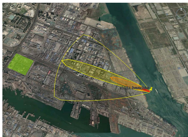
Figure 3. Nitrogen oxides concentration map in the port area 图 3. 港区氮氧化物浓度分布图
