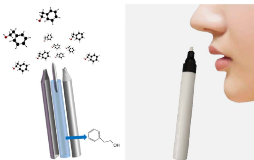
Figure 1. Schematic diagram of odor reference material emission and sniffing
