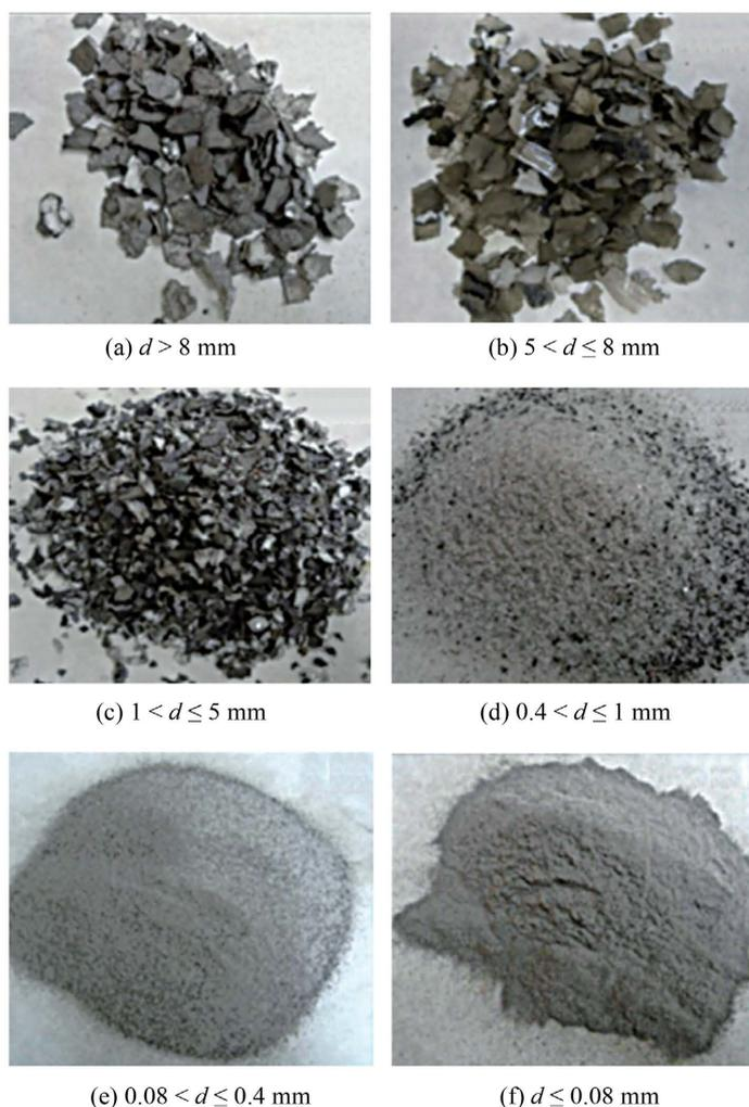
**Figure 2.** After crushing, the materials separated from the filter screen with different diameters  $d$
