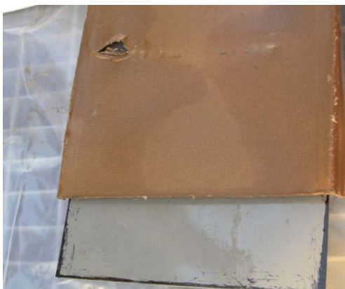
Figure 8. The fifth block of low pressure side oil tank magnetic shielding insulator paper is damaged
