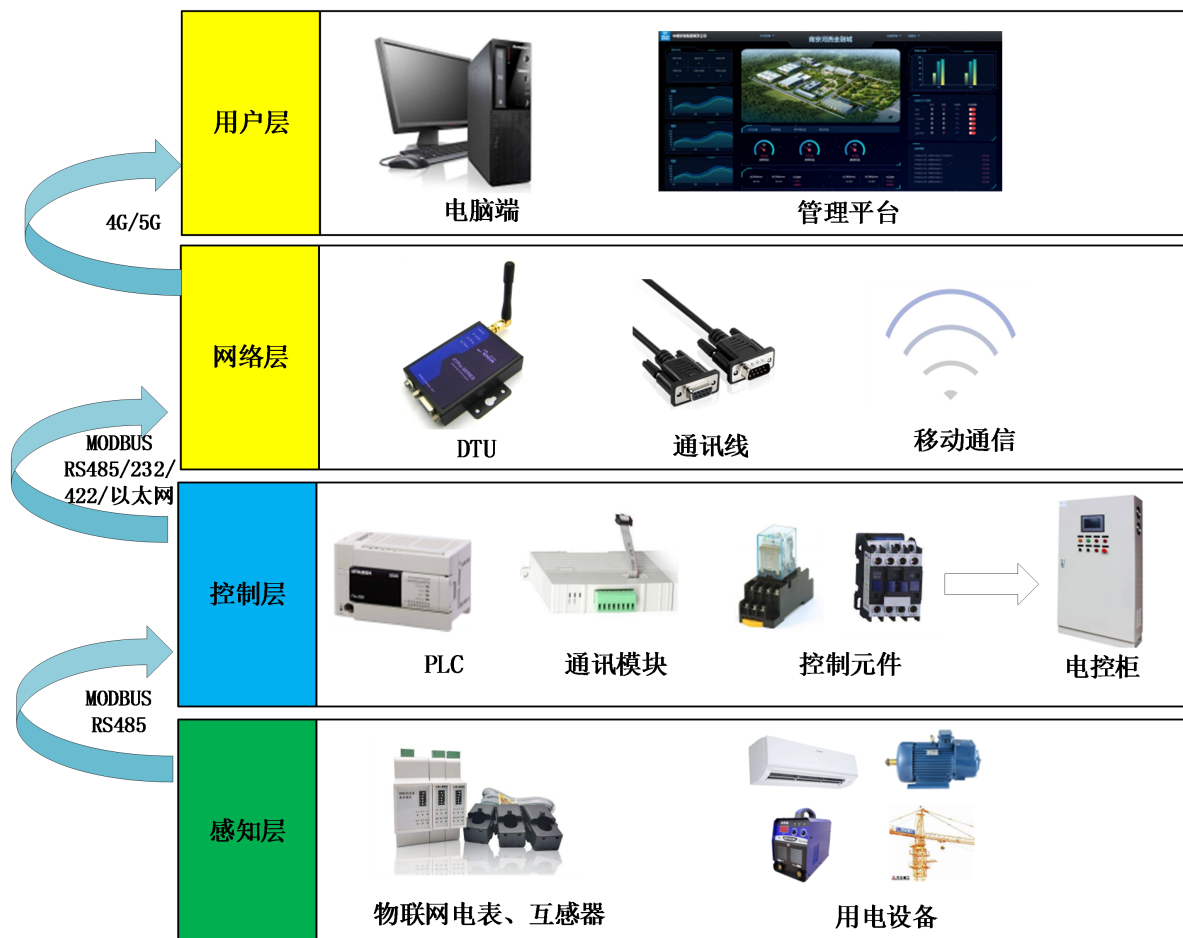
Figure 3. Remote data acquisition system architecture
