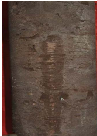
Figure 6. Sepia-colored shaly sandstone from P_3W^1 , 2704.1m in W1 Well
