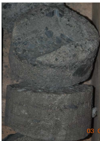
Figure 2. Taupe pebbly coarse sandstone from P_3W^1 , 2385.1 m in W2 Well
