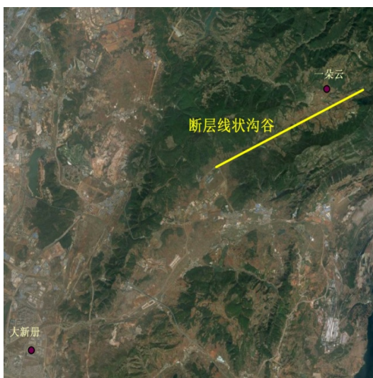
Figure 6. F4 fault and valleys with linear characteristics
