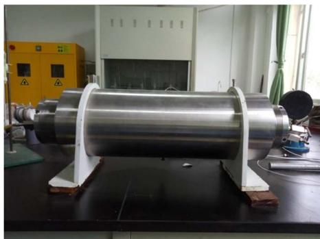
Figure 7. Directional permeability core holder
