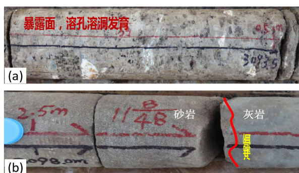
Figure 2. Exposure surface and scour surface on the core for A oilfield 图 2. A 油田岩心上暴露面及冲刷面标志
