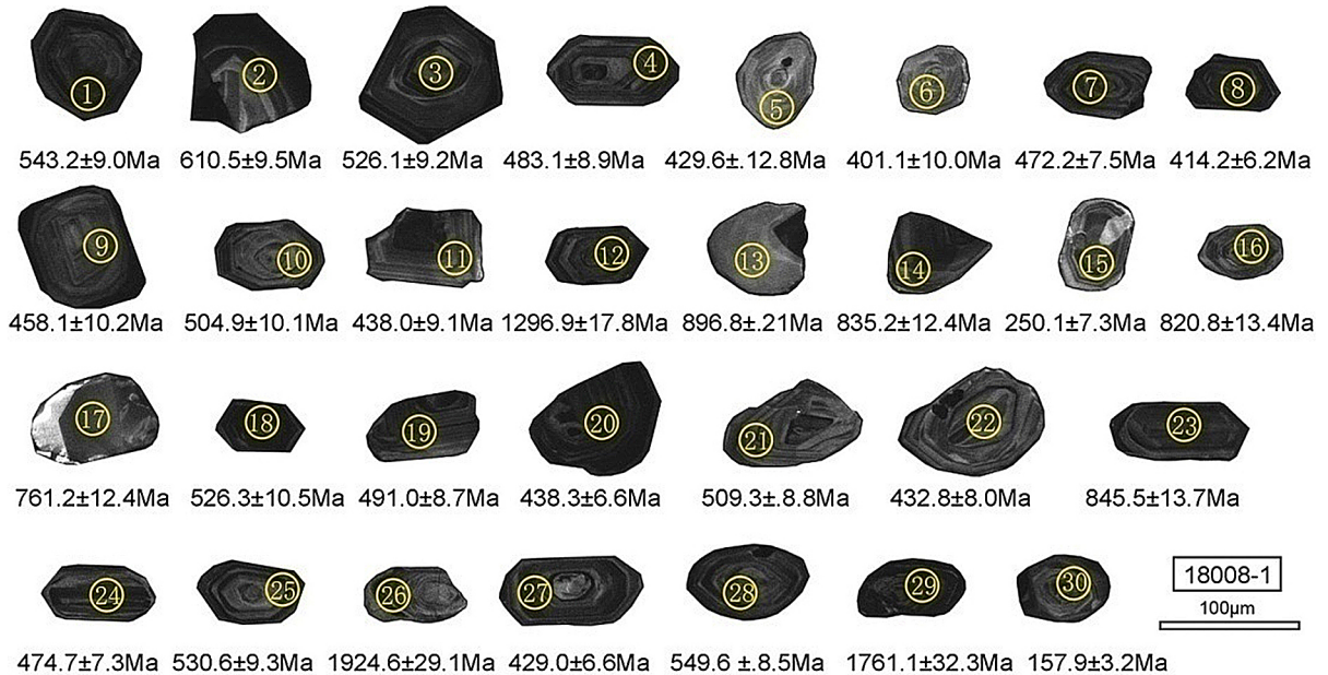
Figure 9. Cathodoluminescence image of metamorphic andesite zircons in Yongxin gold deposit [2]
