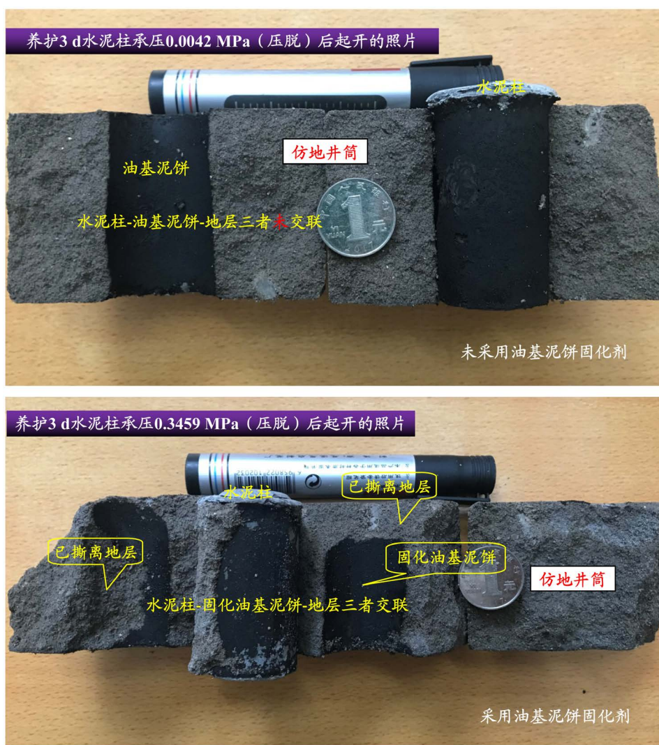
Figure 2. Comparison of cementation at cement-formation interfaces before and after the use of GOS
