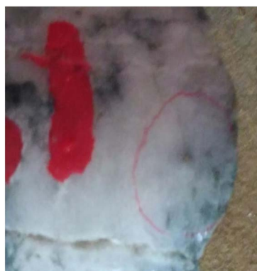
Figure 9. Coarse-grained AU in Quartz vein of the ZK0410 core 图 9. ZK0410 岩心上石英脉中见粗粒明金
