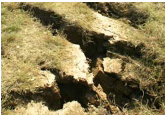
Figure 1. Seismic subsidence disaster of collapsible loess
