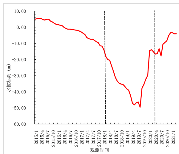
Figure 5. Dynamic change of water level in No.9 observed hole of C_3I aquifer 图 5. 九 C_3I 孔水位动态变化
