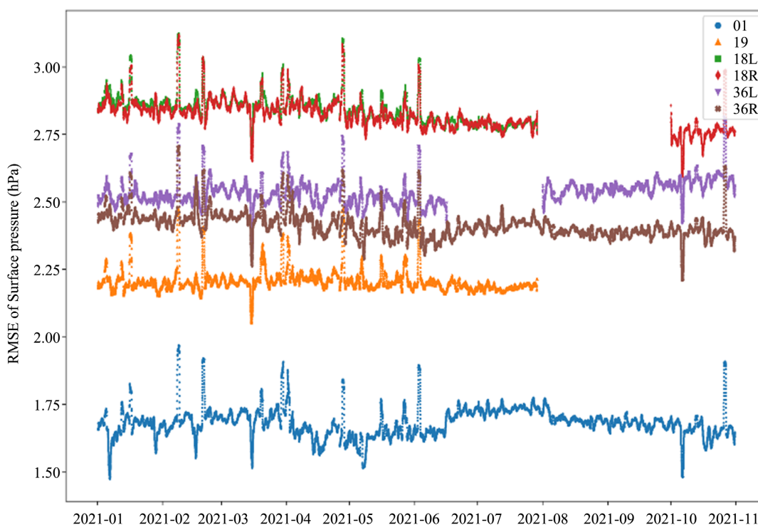
Figure 1. Time series of root mean square error of air pressure at 6 points in Capital Airport
