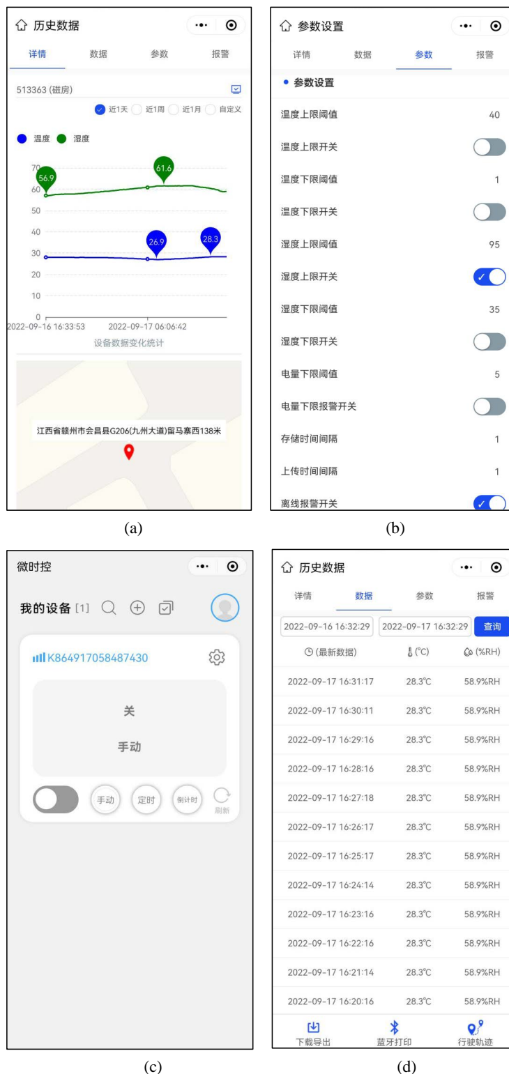
Figure 2. Some functions of intelligent temperature and humidity switch: (a) Temperature and humidity data change; (b) Parameter setting of intelligent temperature and humidity platform; (c) Intelligent switch control; (d) Real time monitoring data of intelligent temperature and humidity platform
