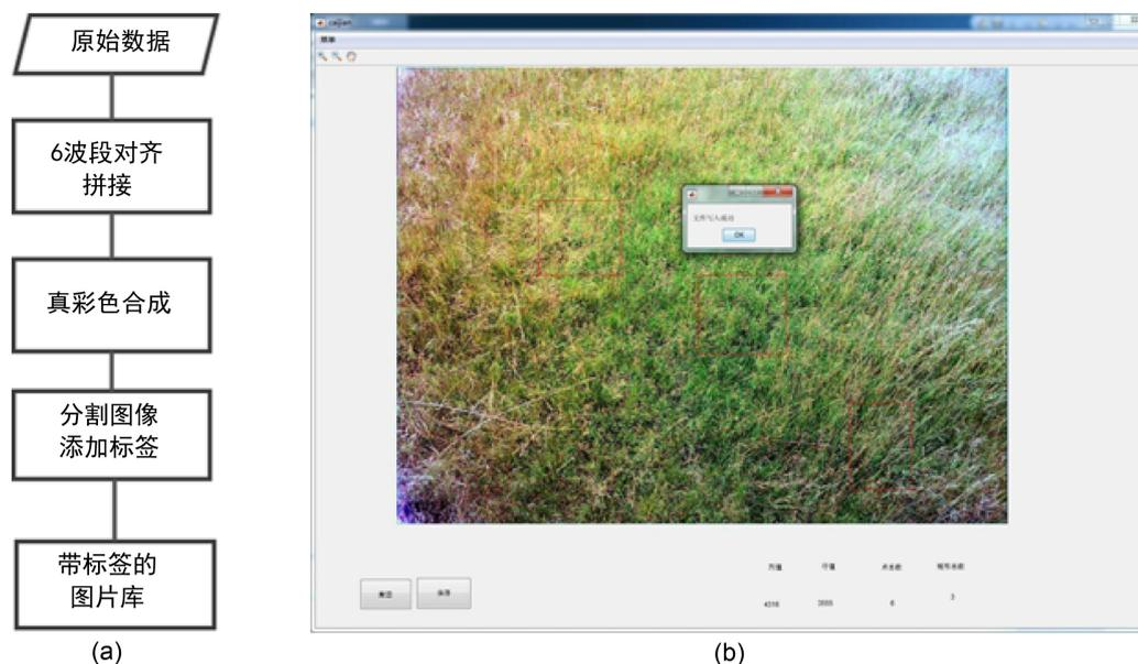
**Figure 5.** The construction method of database with labeled plant samples (a): tagging plant sample database construction flow chart; (b): image acquisition and tagging software developed by laboratory
