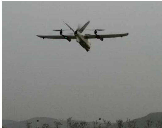
Figure 4. Quadrotor to fixed wing conversion step 图 4. 四旋翼-固定翼转换阶段
