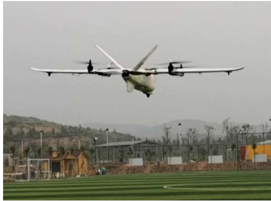
Figure 3. Takes off vertically by Quadrotor 图 3. 四旋翼垂直起飞
