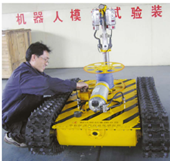
Figure 1. For Anshan Kaixin company and Shenyang Research Institute of Chinese Academy of Sciences jointly develop tracked rescue robot
