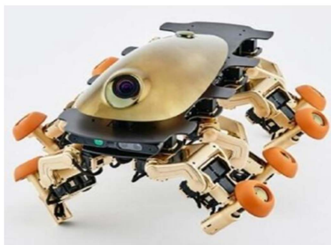
Figure 6. The wheel legged robot is developed for the future robotics research center of Chiba University of technology in Japan 图 6. 日本千叶工业大学的未来机器人技术研究中心研制的轮腿式机器人
