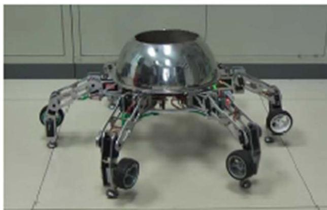
Figure 5. A six wheeled legged robot was designed for Xu Kun and others 图 5. 徐坤等设计了六轮腿式机器人
