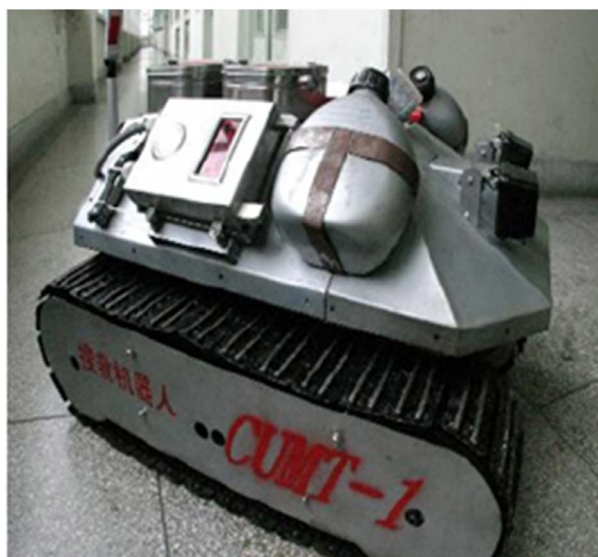
Figure 2. It is the first tracked coal mine search and rescue robot developed for the Research Institute of China University of mining and technology
