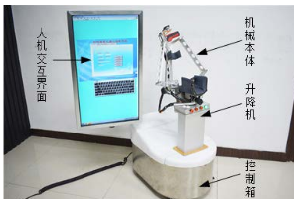
Figure 2. Prototype of the third generation elbow and wrist rehabilitation robot 图2. 第三代肘腕康复机器人样机
