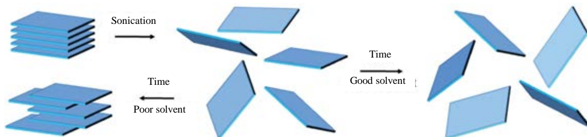
Figure 6. The influence mechanism of solvent molecules to prepare g\text{-C}_3\text{N}_4 nanosheets with liquid exfoliation method 图 6. 液相分离法制备 g\text{-C}_3\text{N}_4 纳米片时溶剂的影响机理
