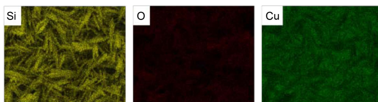
Figure 8. EDX area scan of the sample with Si deposition time of 30 min
